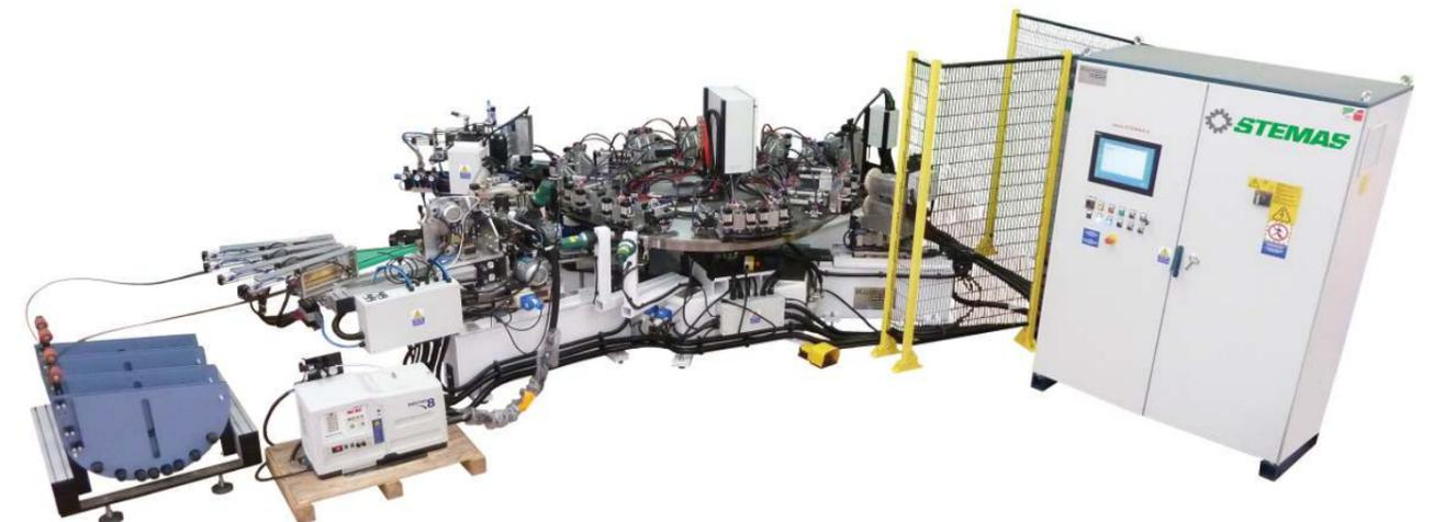
**ROTARY** EST UN CENTRE D'USINAGE AVEC PALETTE ROTATIVE, PERSONNALISABLE POUR DIFFERENTS PROCESSUS DE TRAVAIL : PLACAGE, AFFLEURAGE, POLISSAGE, FRAISAGE ET PONCAGE
