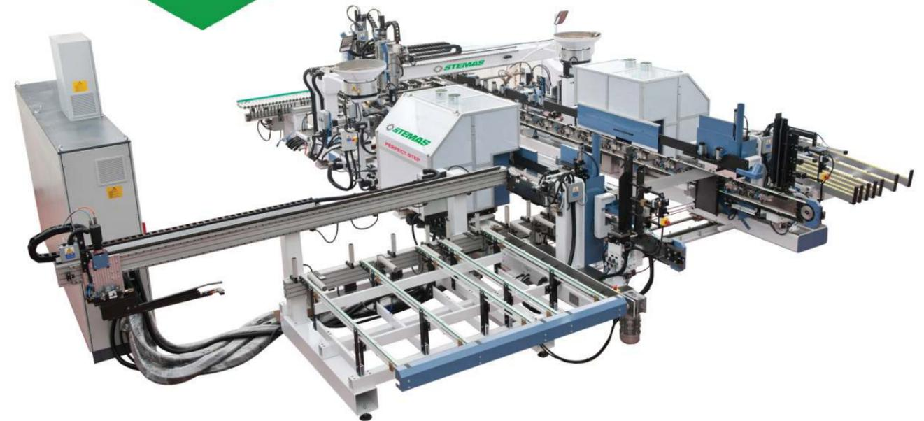
**PERFECT-STEP** EST LA MACHINE ENTIEREMENT PERSONNALISABLE POUR LA COUPE A 90° ET 45°, LE FRAISAGE, LE CHAMFREINAGE, LE PLACAGE, L'AFFLEURAGE, L'ESTAMPAGE DE FILM, LE PERCAGE, L'INSERTION TOURILLONS ET LE PONCAGE
