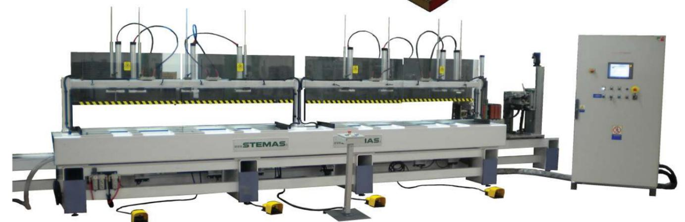
**WAVE** EST LA SOLUTION POUR LE PLACAGE ET L'AFFLEURAGE DE PIECES COURBES, AVES 2 OU 4 AXES CONTROLES
