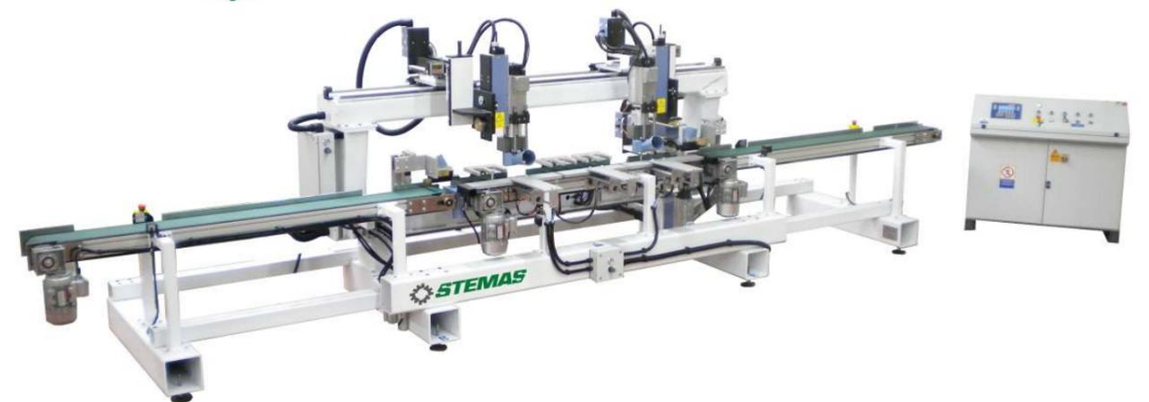
SOLUTIONS PASSANTES POUR LE PERCAGE ET LE FRAISAGE D'ELEMENTS POUR FENETRES
