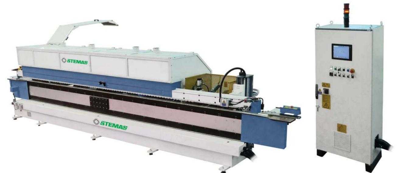
**SLIDE** EST LA SOLUTION DE PLACAGE POUR PIÈCES ÉTROITES DE 30mm
