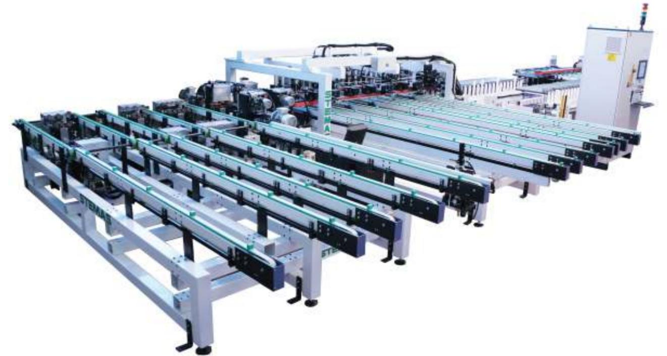
ENSAMBLAJE DE LAS TAPETAS AL ELEMENTO CENTRAL USANDO COLA PUR O HOT-MELT
